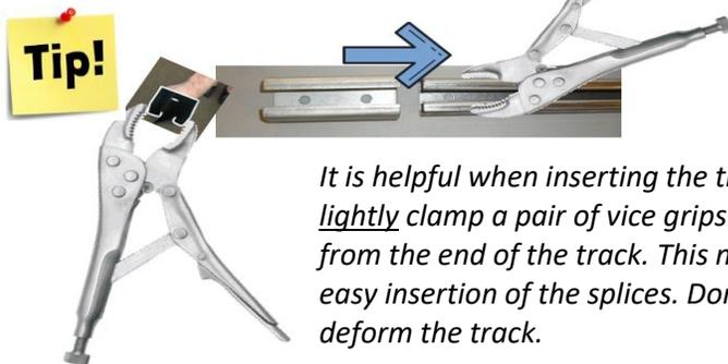
*It is helpful when inserting the track into the splices to lightly clamp a pair of vice grips onto the track about 4" from the end of the track. This narrows the track and allows easy insertion of the splices. Don't pinch too hard or you will deform the track.*
